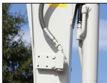
Auxiliary Hydraulic Lines
