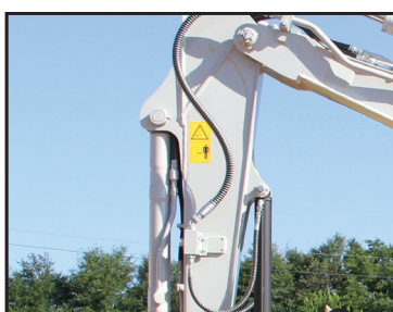
Auxiliary Hydraulic Lines
