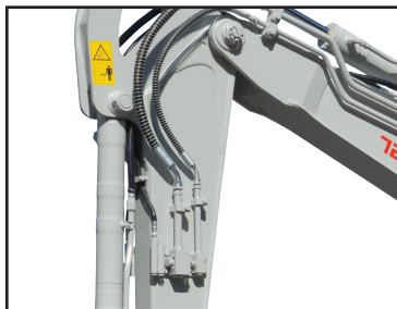
Auxiliary Hydraulic Lines
